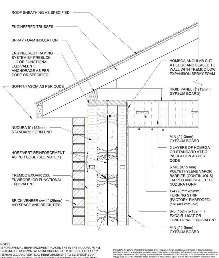
MULTIPLES OF 8" (203mm) O.C. REFER TO NUDURA REINFORCEMENT PLACEMENT DETAILS. Combustible Construction
